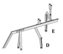
Take one of the Cones Part 'F' and attach it to the Part 'D' using big Bolt provided as shown in the diagram. Similarly attach the other Cone Part 'F' with Part 'E' in opposite direction using the big Bolt provided.
