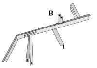
Attach the flat shaped base of Part 'C' on top of main angle frame using the Nuts and Bolts provided. This has the other 'U' shaped support already fixed for attaching handle.
