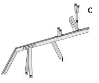
Now take Part 'D' and Part 'E' which have a big nut welded on one end and a pin on the other end. Attach Part 'D' with the help of the nut and bolt provided to the slotted angle welded on the main angle frame of the weeder. Likewise attach Part 'E' on the other slotted angle welded on the main angle frame. Please note that Part 'D' and Part 'E' are mirror images of each other.
